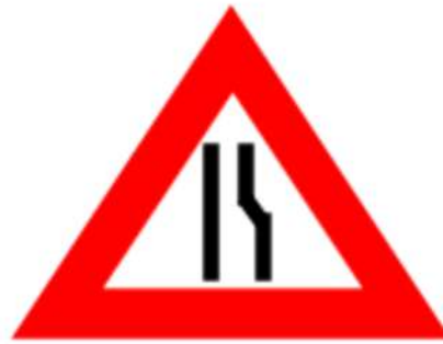
Road narrows on right-hand side ahead
