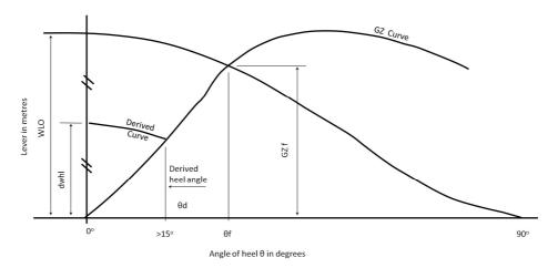
**WLO** is the magnitude of actual wind heeling lever at  $0^{\circ}$  which would cause the vessel to heel to the 'down flooding angle' ( $\phi_f$ ) or  $60^{\circ}$  whichever is the least.
